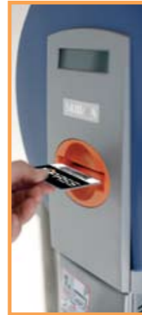
The card readers accept most card and ticketing systems, including Print@Home and RFID. Anti-passback software prevents double use of tickets.
